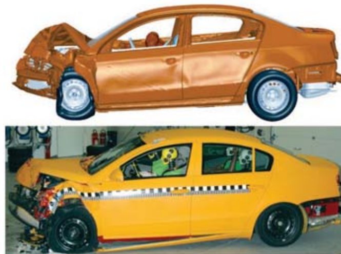
Fig. 4. The comparison of virtual and real frontal impact test [8]
